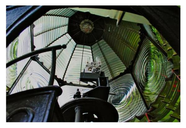
The Pensacola Lighthouse is equipped with one of only thirteen working First-Order Fresnel (fruh-NELL) lenses in the United States. Our lens was cut and polished by Parisian lens-maker Henry Lepaute. Standing over 10 feet tall and 6 feet wide, it contains 344 hand-cut prisms. Its eight bulls-eyes focus the light into bright beams that can be seen 27 miles out to sea. Every lighthouse has a light signature, or *characteristic* (see below); ours is a white flash every 20 seconds.
